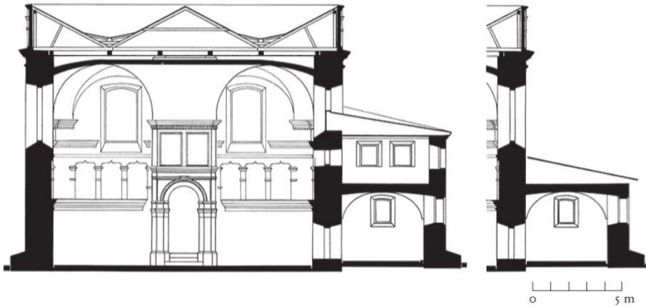
227. Longitudinal section looking towards the *bimah*, after reconstruction
